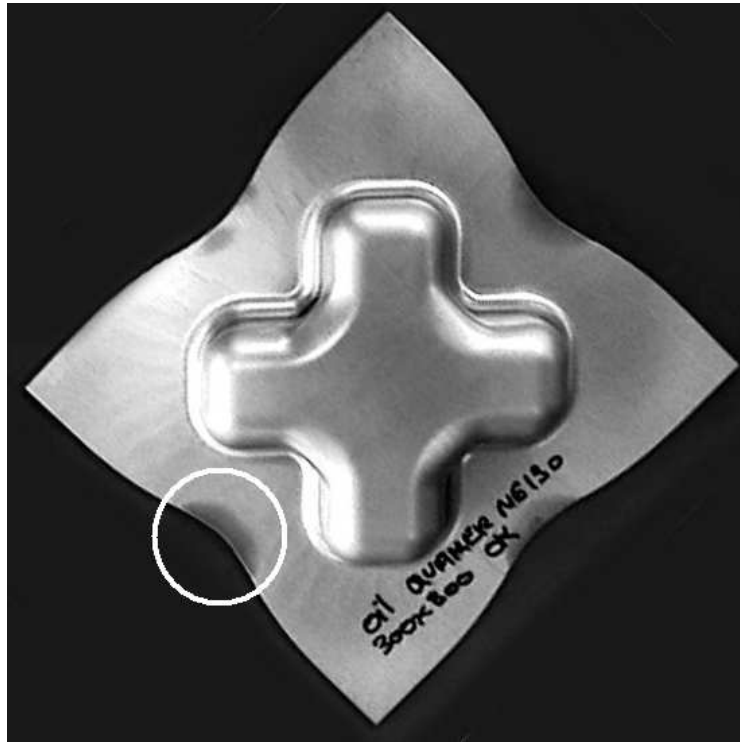
Figure 2.6: Shiny spots on the blank reveal high-pressure zones (picture courtesy of Corus RD&T)
